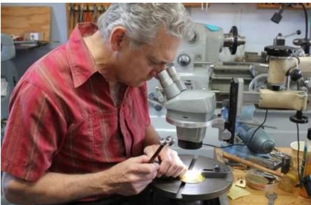
Joe LaCour engraving the micrometer plate
