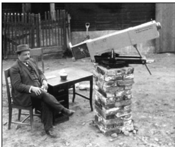
Fig. 4: Tadeusz Banachiewicz and his chronocinematograph in 1932. Note the dire state of the courtyard and the ad hoc arrangement of a pile of bricks for a telescope mount. A spade in the background hints at work in progress. (The Jerzy M. Kreiner private collection, CC BY-NC-ND 4.0)
