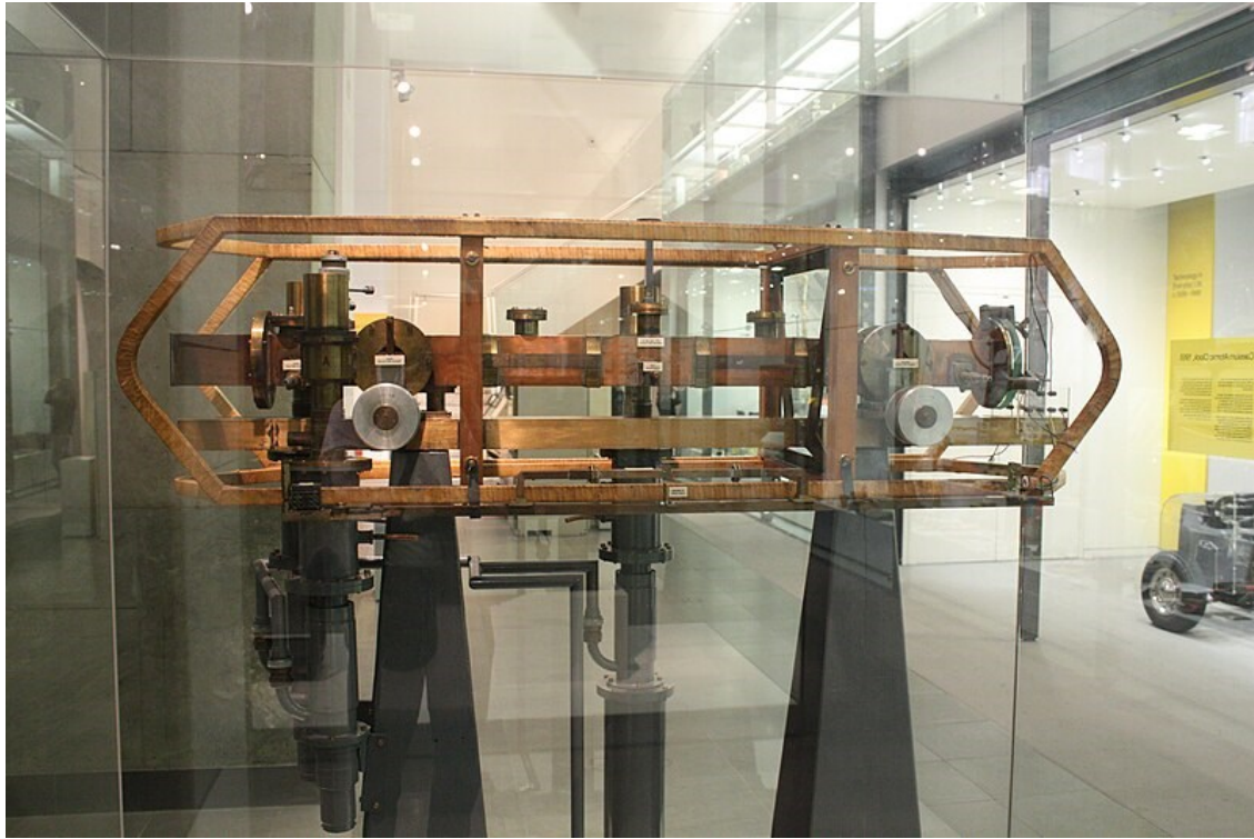
Figure 1: Mk. 1, the first caesium atomic clock from the National Physical Laboratory (NPL) in London from 1955, on display in the Science Museum in London (Wikimedia Commons).
